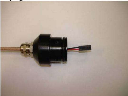
Unscrew the cable grip from the case's lower section
