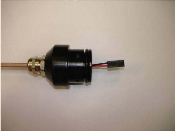
Plug in the inline connector. Slide the Circuit board back in the slots and push the case back together. Take care that the o-ring is inserted correctly.
