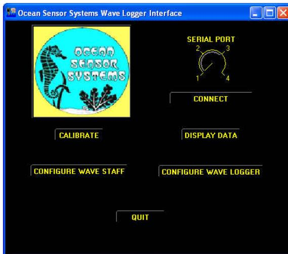
3. Select the serial port (typically #1) then click the CONNECT button. You should see a new window stating that you have successfully connected.
