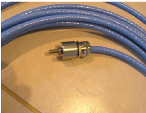
The tensioning should not exceed 10lbs though the unit is designed to take up to 100lbs. This will allow for dynamic loading due to the wave forcing without exceeding the maximum allowable load. In addition, intermediate supports may be used along the length of the cable. The supports should cover as little of the vertical section of the staff as they will create distortion in the measurements. The supports should hold the cable
