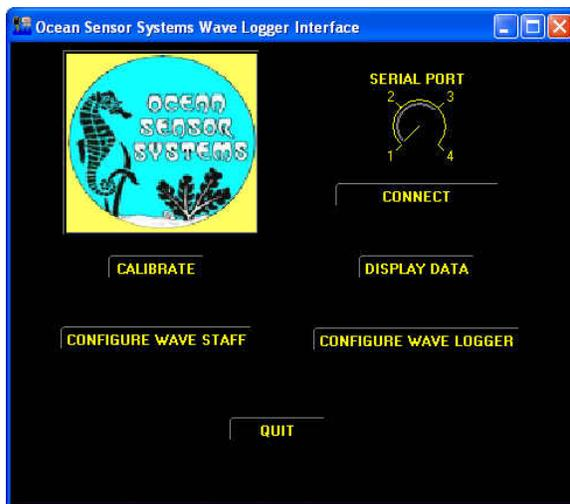
3. Select the serial port (typically #1) then click the CONNECT button. You should see a new window stating that you have successfully connected.
