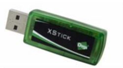
The XStick USB Adapter XU-Z11 part #OSSI-581-016 for US,CA,EU with a RF Line of Sight Range of 66 ft. and Indoor/Urban Range of 200 ft.
