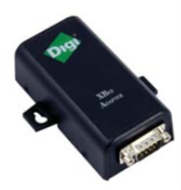
XBee RS232 Adapter XA-Z14-CS2PH part #OSSI-581-020-A Pro for North America with a RF Line of Sight Range of 2 miles and Indoor/Urban Range of 300 ft. and OSSI-581-020-W Pro for International with a RF Line of Sight Range of 4000 ft. and Indoor/Urban Range of 200 ft.
