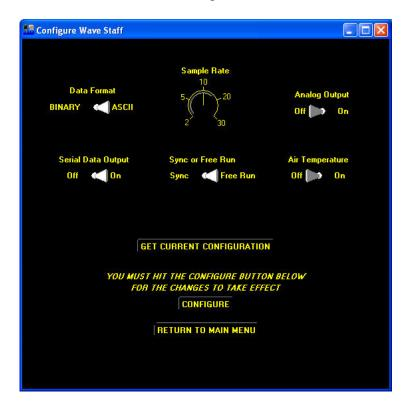
Make sure the settings are configured: Set Data Format to ASCII Set Water Temperature to off Set Serial Data Output to On Set Sync or Free Run to Free Run
